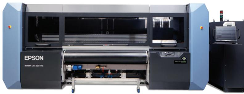
Monna Lisa Evo Tre is an industrial digital textile printer based on Total Solution, the fully integrated system where all components belong to the same process to guarantee the best printing results and the utmost customer satisfaction. This is the result of the synergy of Epson inkjet printing technology with engineering by F.Ili Robustelli and pre/post-treatment and inks by For.Tex, both companies now part of the Epson Group.
